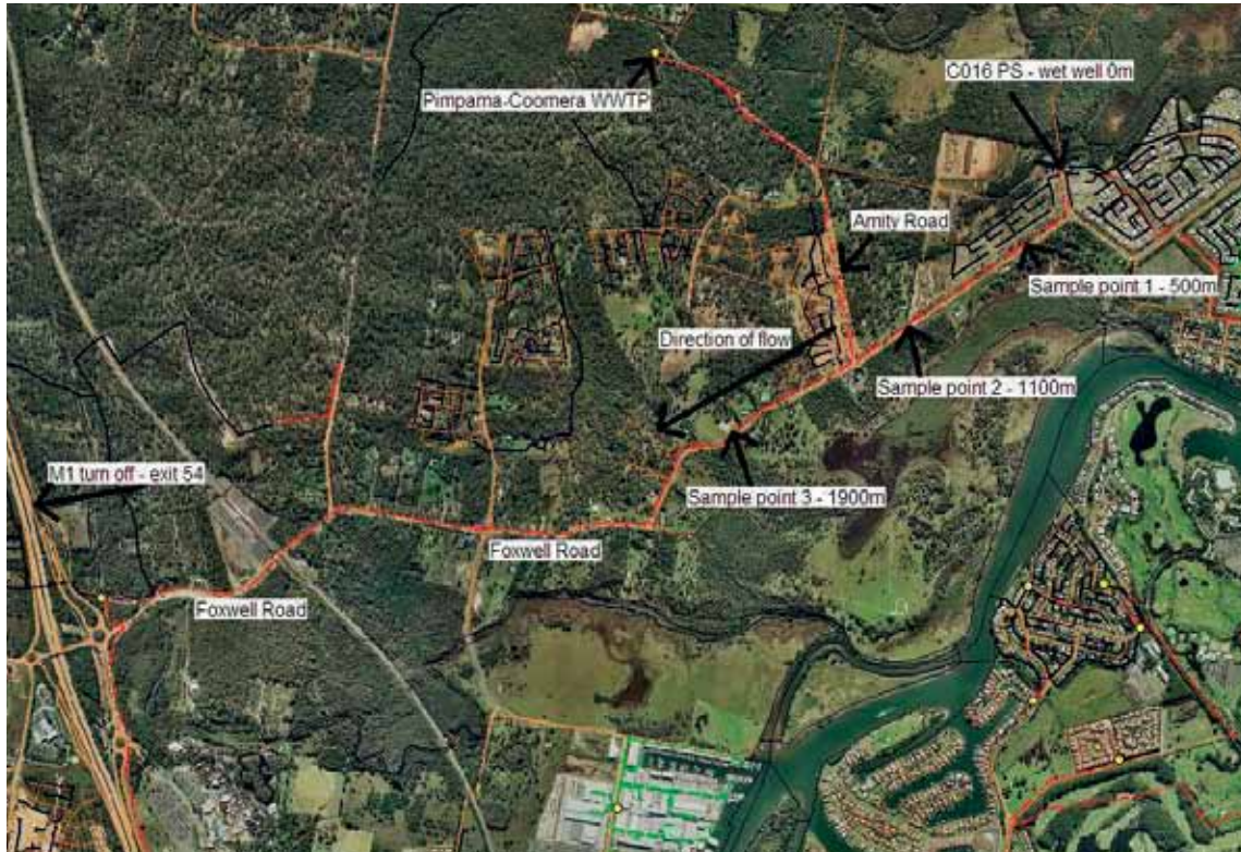
FIGURE 23 AERIAL PHOTOGRAPH OF THE C016 RISING MAIN. SAMPLES WERE COLLECTED FROM THE C016 PUMP STATION WET WELL (0 M), SAMPLE POINT 1 (AT 500M), SAMPLE POINT 2 (AT 1100M) AND SAMPLE POINT 3 (AT 1900 M)
